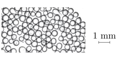
Shear-thickening potato starch in water
